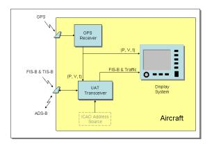
The aircraft architecture (illustrated above) will consist of two basic configurations:
