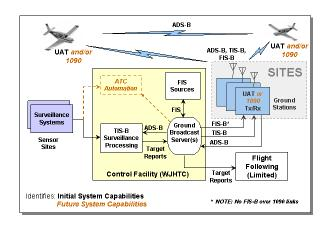
Future new broadcast services products are possible, since the architecture supports expansion without avionics hardware changes. Future enhancements are expected to use the same "signal in space" technology offering graphical Temporary Flight Restrictions (TFRs) and Special Use Airspace (SUA) as well as other graphical and weather products.
